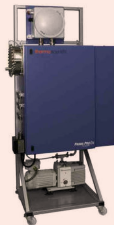
Figure 5: Prima PRO Ex Hazardous Area Process MS.
