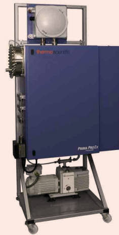
Figure 5: Prima PRO Ex Hazardous Area Process MS.
